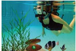
Underwater treasure quest: As a demonstrator Fraunhofer FIT created the world's first mobile underwater AR game. Its main component is a waterproof display in front of a diver's mask. The display lets the diver see his or her real underwater environment plus additional virtual objects.
